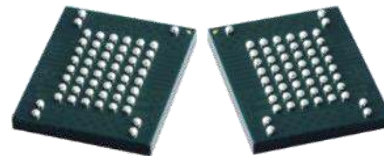
Lead-Free → Leded BGA Reballing
